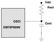
Fig. 34. External RC Oscillator Mode Circuit
